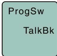
**TalkBk** is a “push to talk” function that is active only while the button is pressed. The talkback function provides a communication channel when used with a receiver equipped with this function, such as a Venue Wideband receiver with firmware
