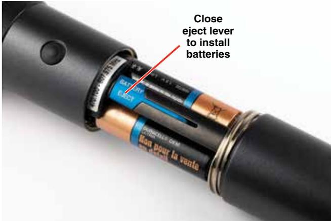
The contacts are very tight to prevent the batteries from “rattling” as the transmitter is being handled. Pull the eject lever outward to remove the batteries. The battery tips will move outward, making them easier to grasp.
