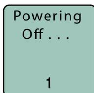
**NOTE:** If the Power Button is released before the countdown is completed, the unit will remain turned on and the LCD will return to the same screen or menu that was displayed previously.
