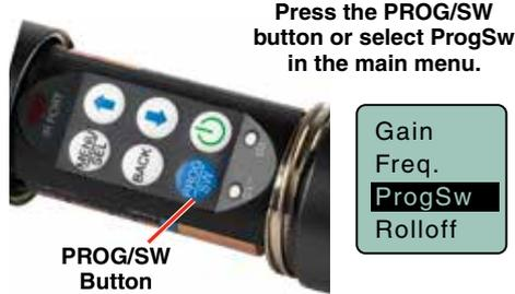
The **ProgSw** menu provides a scrollable list of the available functions. Use the UP/DOWN arrows to highlight the desired function and press BACK or MENU/SEL to select it and return to the main menu.
