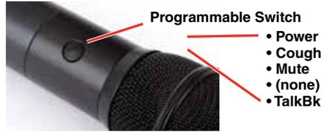
The **ProgSw** button on the keypad opens a setup screen to select the programmable switch function. Enter this setup screen and then use the UP/DOWN arrows to select the desired function and press the MENU/SEL button to return to the Main Window.
